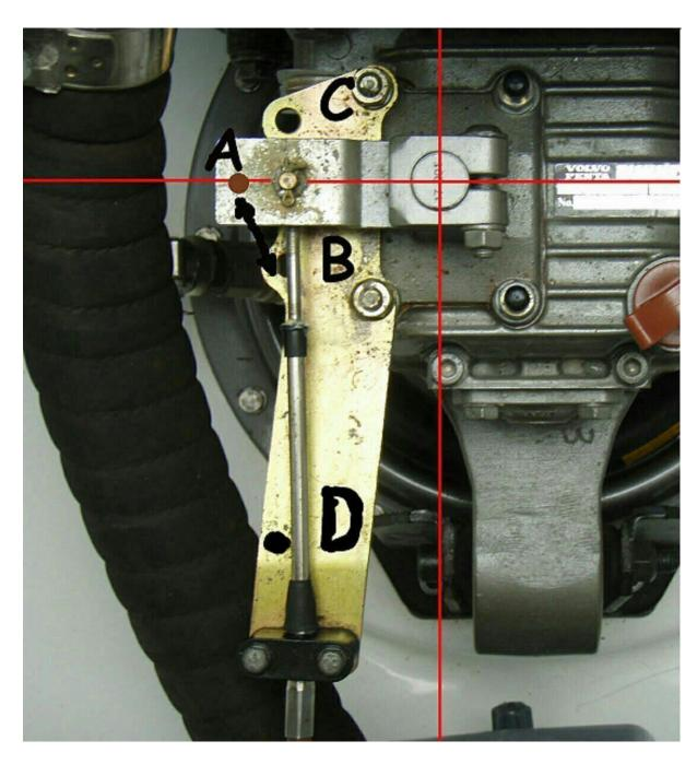
3. Further example of setup on unknown engine. One can see a simulation of the future leaded cable made with a simple cable to test the two positions of neutral and reverse.
