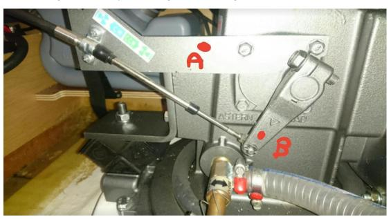
2. Arrangement for Volvo engine. The image should represent the neutral position. Holes "C" and "B" would appear to be already present. Creating a new hole in "A".
