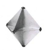
RADAR REFLECTOR OSR reference 4.10 Radar reflector: octahedral (with plates circular 12" or rectangular 16") or of min 2m<sup>2</sup> radar cross-section.
